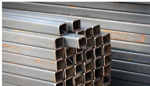
Fig:2.2.1 Hollow Square Pipe
