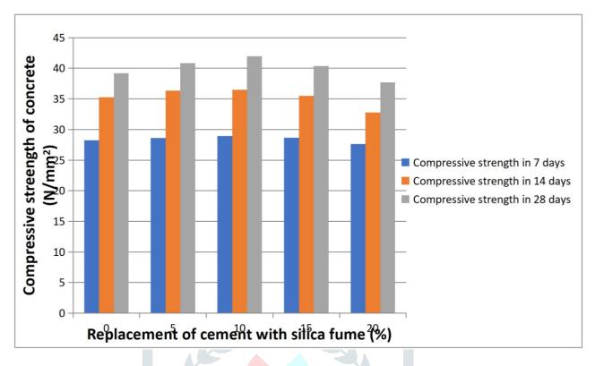
Compressive strength of M30 grade of concrete increased for 5%, 10%, replacement of cement with silica fume. As we increased further replacement of cement 15%, 20%, compressive strength of M30 grade concrete starts decreasing.
