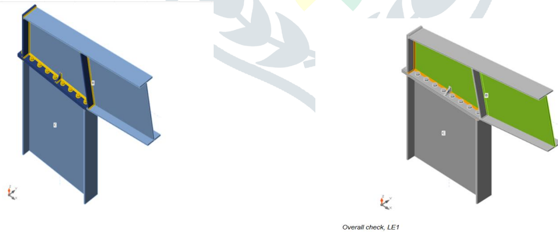
Fig. 2. Bolted connection between rafter and column This all images are taken from idea static report for overall check, strain check and stress check for load check.
