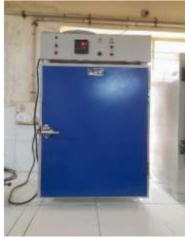
Figure 3: Hot air oven
