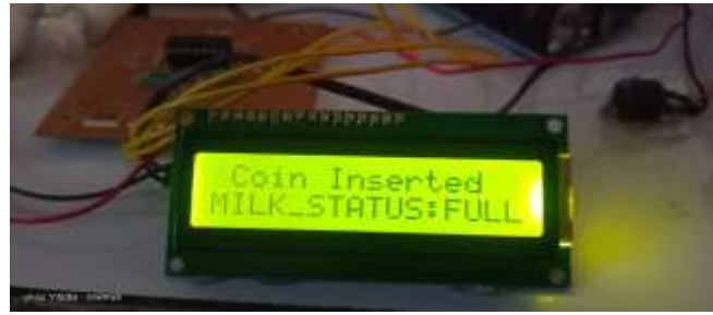
Fig 4 LCD output After inserting a coin
