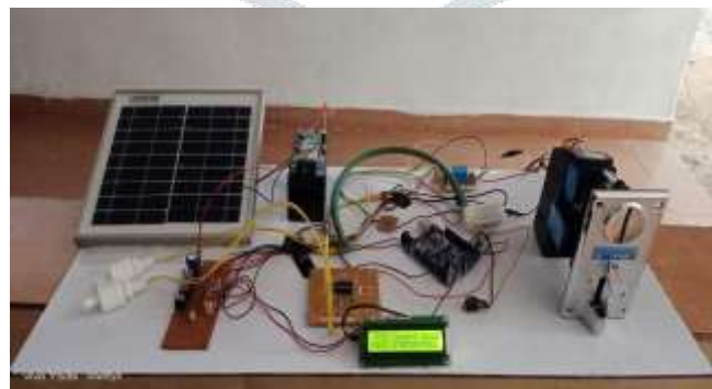
Fig 2 Project Kit (solar-coin Based Milk Dispensing system)
