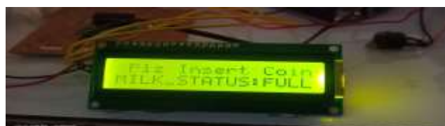
Fig 3 LCD output before inserting a coin
