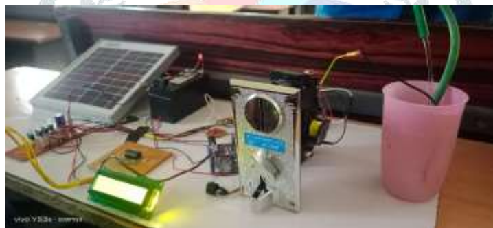
Fig 6 Dispensing kit output After inserting a coin
