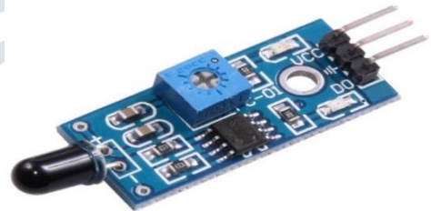
Fig- 4 Fire Detection Sensor
