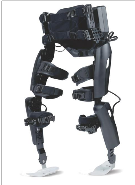
Fig 6: ReWalk, wearable exoskeleton designed to provide powered assistance to facilitate walking. Source [8]
