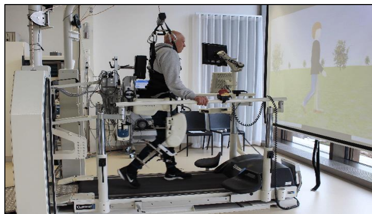
Fig 1: The Lokomat (Hocoma) is a bilateral gait robotic orthosis that uses body-weight support and controls the patient's leg movements. Source [5]
