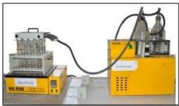
Figure 2.6.3 Digestion Unit Plate
