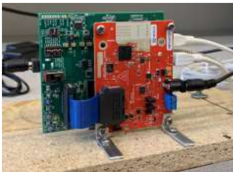
Fig.3(a): FMCW radar test-bed (red board: AWR1642 BOOST; green board: DCA1000 EVM)
