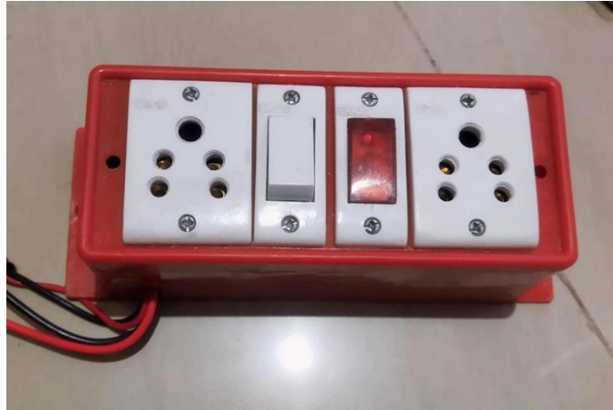
Figure 2.1 - 2 Sockets, 1 Switch and 1 Indicator Light Setup connected to the CFL Driver Inverter Circuit
