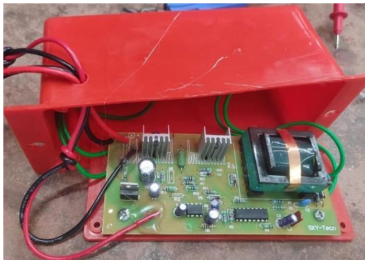
Figure 2.2 - CFL Driver Inverter Circuit
