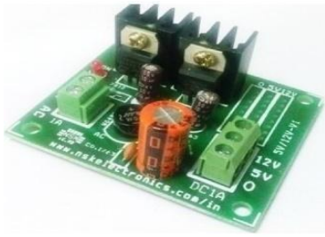
Fig: 1. Power supply unit
