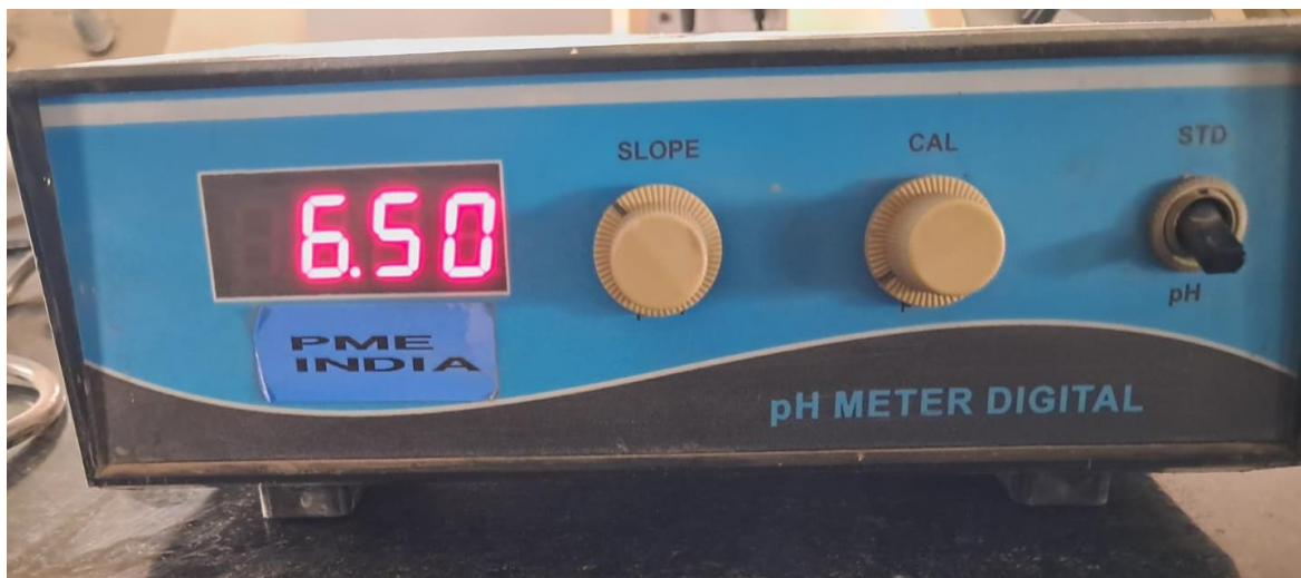
Fig.12:- Testing of pH of antidandruff gel by using digital pH meter
