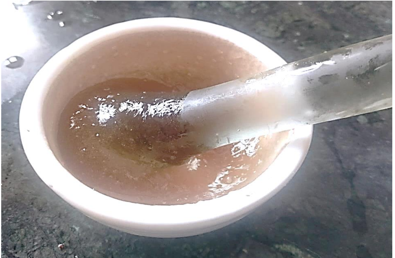
Fig.10:- Agitating gel in mortar pestle
