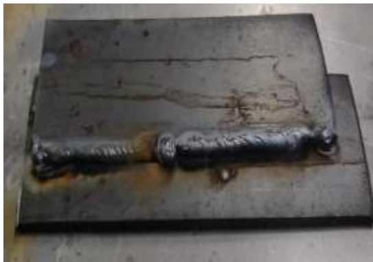
Fig:1.2 Lap Joint
