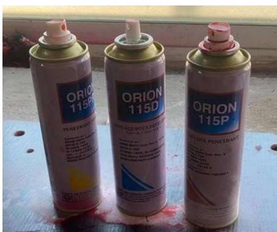
Fig:3.7 Penetration Test consumables
