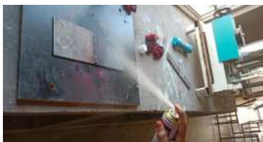
Fig:3.10 Applying Of Developer
