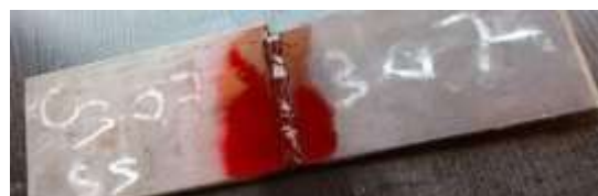
Fig:3.8 Clean the weld joint with penetrant remover
