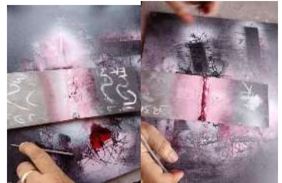
FIG:4.3 defect occurred for stainless steel
