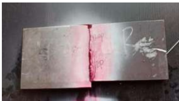
Fig:3.11 Recording the defects
