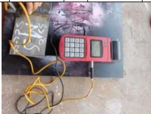
Fig:4.2 Hardness test for ms filler rod welding PENETRATION TESTING
