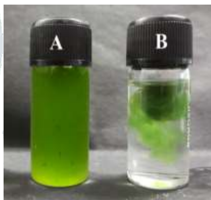
Fig1(c): Bioflocculation of Chlorella sp (A) Control (B) Delonix regia leaf protein at pH 2
