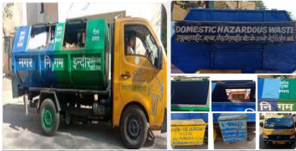
Picture :4 The waste collecting vehicle and its different compartments for waste segregation.
