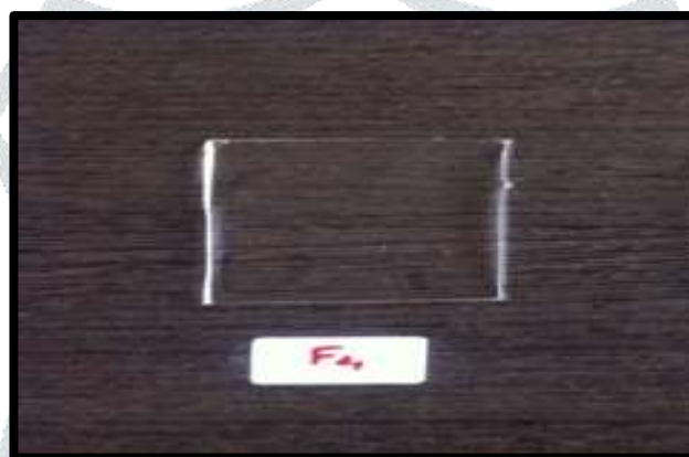
Figure 7: Appearance of FDOFs after removing from glass mold (F4)
