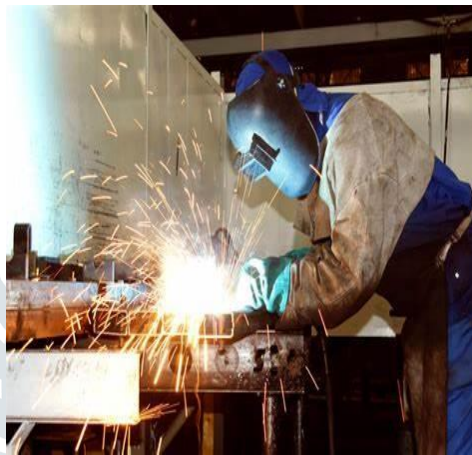
Fig : Arc Welding
