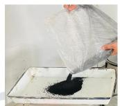
Composition (wt%) Ultimate **Proximate** 53.4 Total carbon Fixed carbon 31.70 Hydrogen 4.0 Volatiles 47.55 Oxygen Moisture 3.01 11.6 Sulfur 0.017 Ash 17.74
