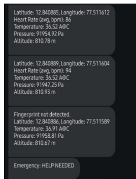
Figure 12: continuous monitoring of data is sent through SMS
