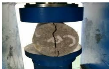
Fig 5.5 Split Tensile strength Test.
