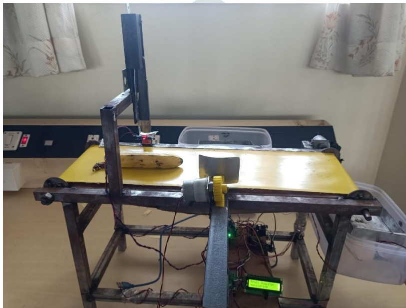
Fig4. Detecting whether the fruit is good or bad.
