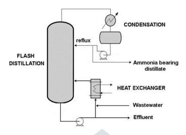
Construction: The production of a flash distillation equipment is proven in Figure 7-7. It includes a pump, that is linked to a feed reservoir. Pump enables in pumping the feed into the
