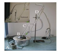
Hydrodistillation the use of the Steam distillation equipment, Clevenger-kind equipment. (A) Power regulator; (B) Heating mantle with spherical backside flask containing water and aromatic leaves; (C) Clevenger-kind equipment that returns the hydrosol to the nevertheless and keeps the crucial oil phase, however best for important oils which might be much less dense than water and consequently float;
