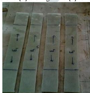
Figure 4.2 [a]: Specimens in "x" direction, [b] Specimens in "y" direction, [c] Specimens in "450" direction.
