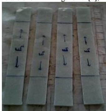
Figure 4.2 [a]: Specimens in "x" direction, [b] Specimens in "y" direction, [c] Specimens in "450" direction.
