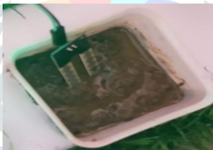
Figure 5: Testing on Wet Soil with Full Of Water
