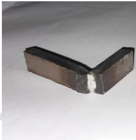
Figure: 8 Impact failure of TIG joint
