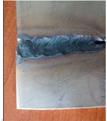
Figure: 3 Butt joint by TIG welding
