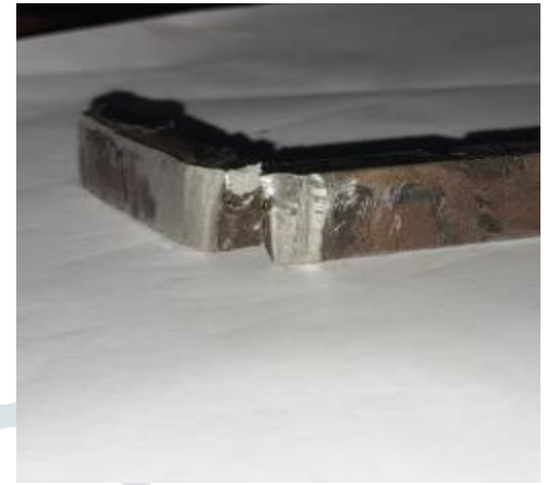
Figure: 9 Impact failure of MIG joint
