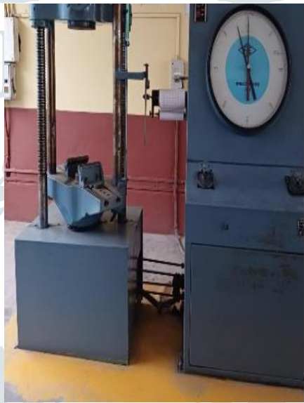
Figure: 5 Universal Testing Machine
