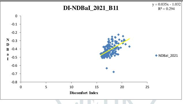
The relation between Discomfort Index and Normalized Difference Built-up Index is given below:
