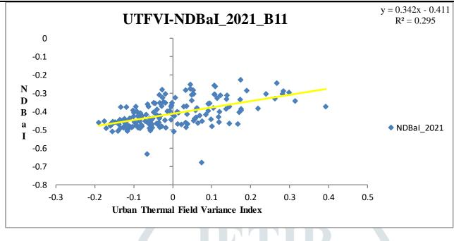
The relation between Urban Thermal Field Variance Index and Normalized Difference Built-up Index is given below:
