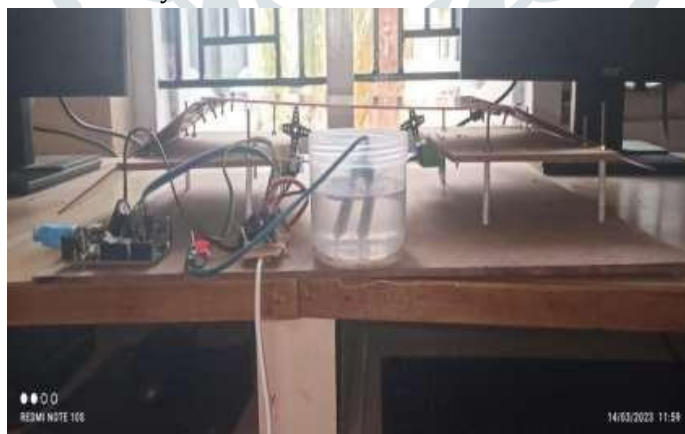
Fig 4: Soil Moisture Sensor detecting Increased water level.
