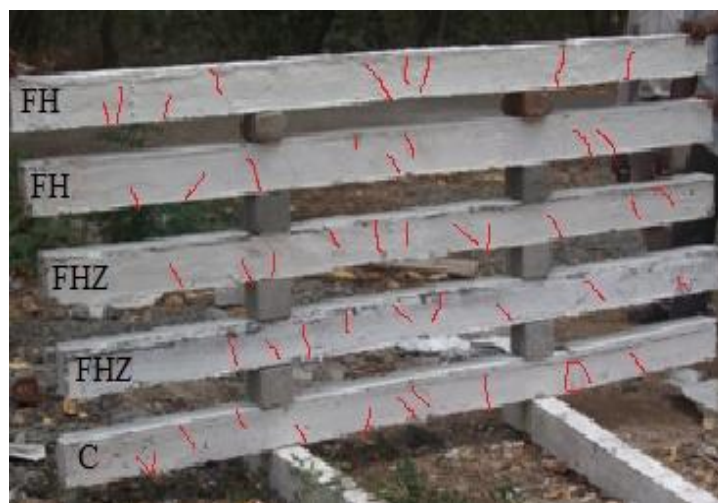
Fig.4.12 Failure pattern for all the beams.
