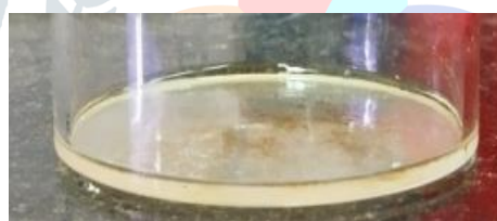
Oil extracted from the stored little millet grain for estimation of peroxide value and free fatty acid.
