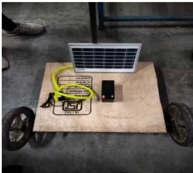
Figure 2.1 Solar-powered fertilizer sprayer model during assembly
