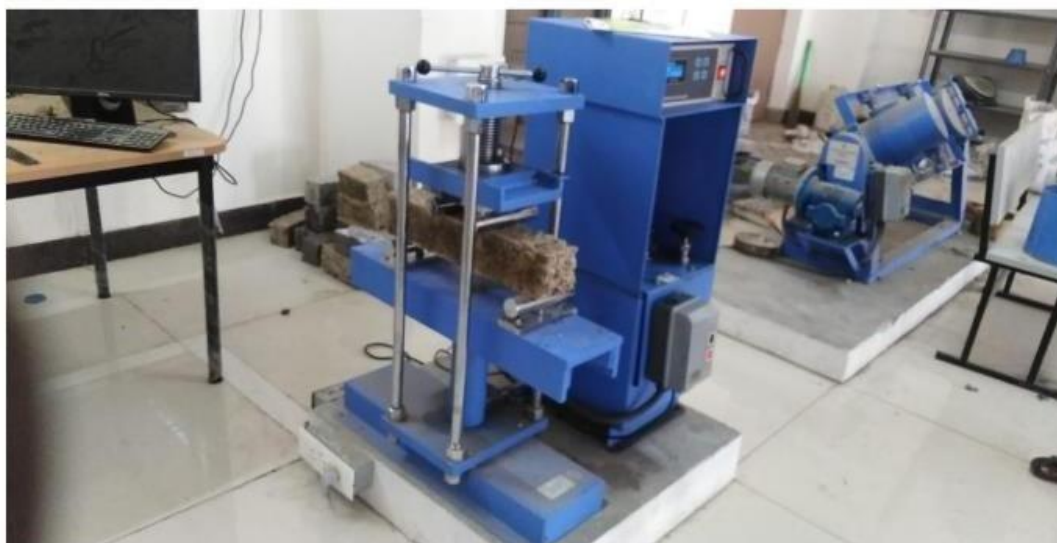
Fig 4.4 Flexural Strength Test
