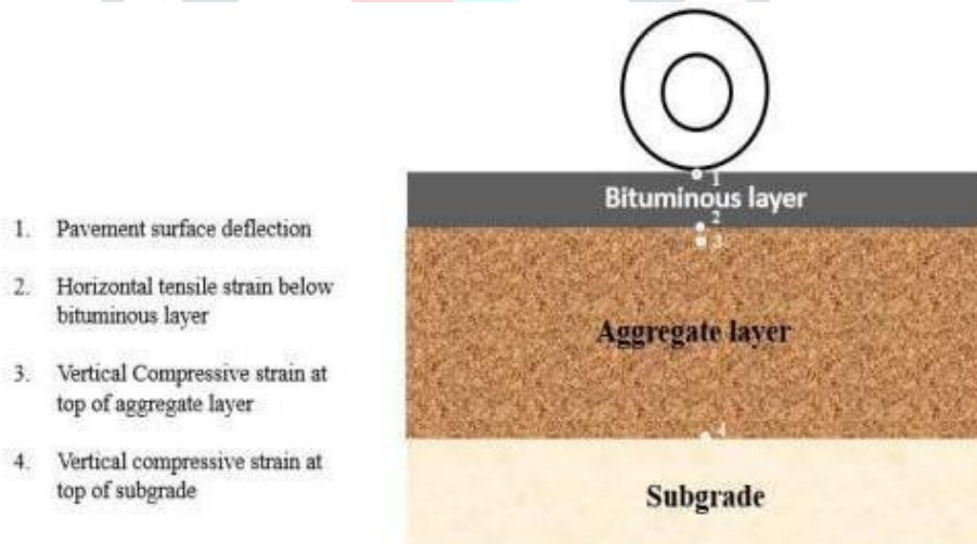
Figure 1.3: Critical Locations of Stresses and Strains in Flexible Pavements
