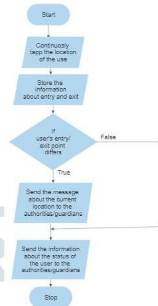
Fig. 5. Flowchart for system on ID card
