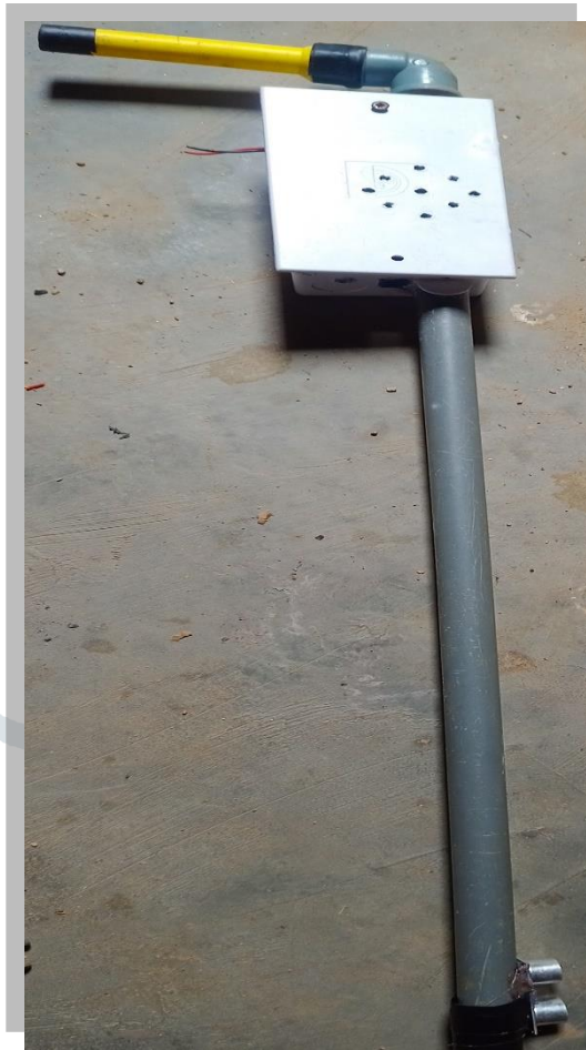
Fig. 9: The implemented blind man stick
