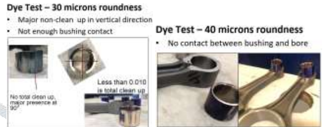
Figure 5: Dye test with 30 microns & 40 microns roundness
