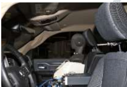
Figure 17: Vehicle Interior Aachen Head & Microphone
