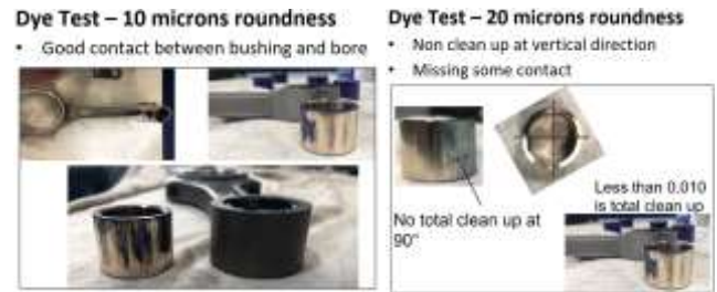
Figure 4: Dye test with 10 microns & 20 microns roundness
