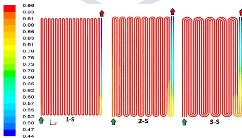
Figure 3.2 H 2 mass fraction distribution in anode channel of PEMFC at 0.5 V
