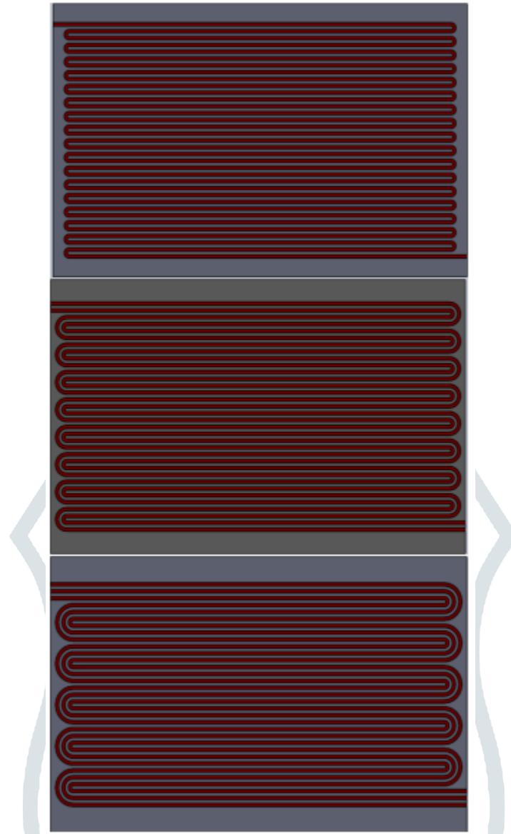
Figure 2.2 7 cm x 12 cm size single (top), double (middle) and triple (bottom) serpentine flow field designs
