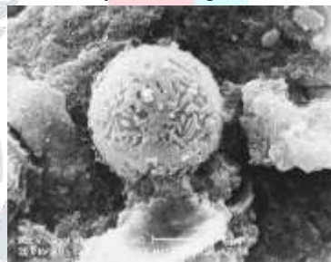
Fig 2.1 CBA particle starting to react with \text{Ca}(\text{OH})_2
