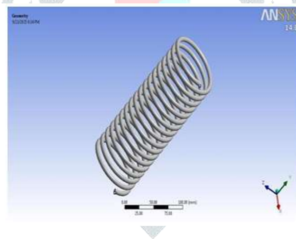
Fig. 2 Spring Geometry model in Ansys
