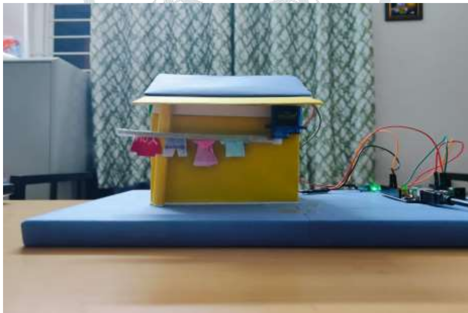
Fig 1: When rain is not detected, cloths are exposed to the outer space.
