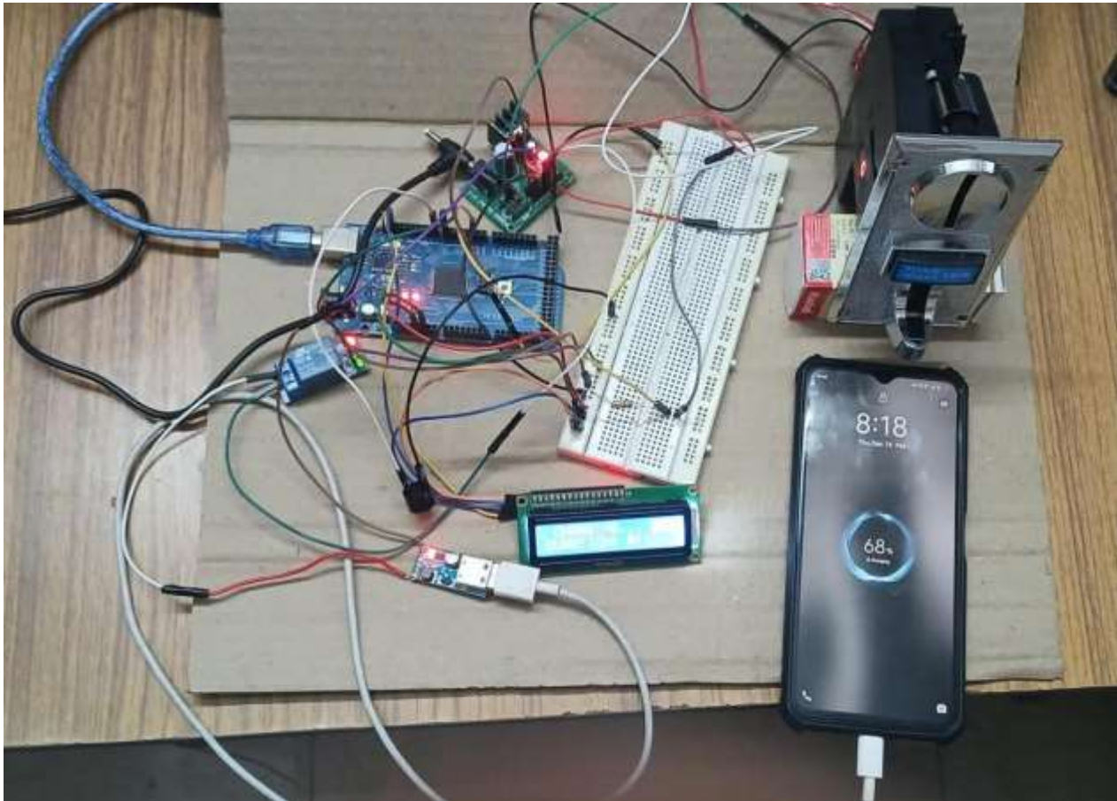
Fig1: Implementation of Mobile Charging Using Coin Insertion
