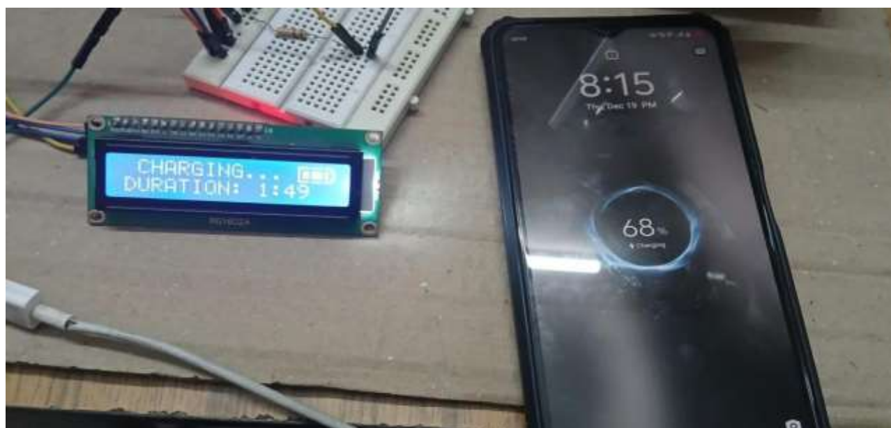
Fig 3: Displaying 'Charging started and time left'
