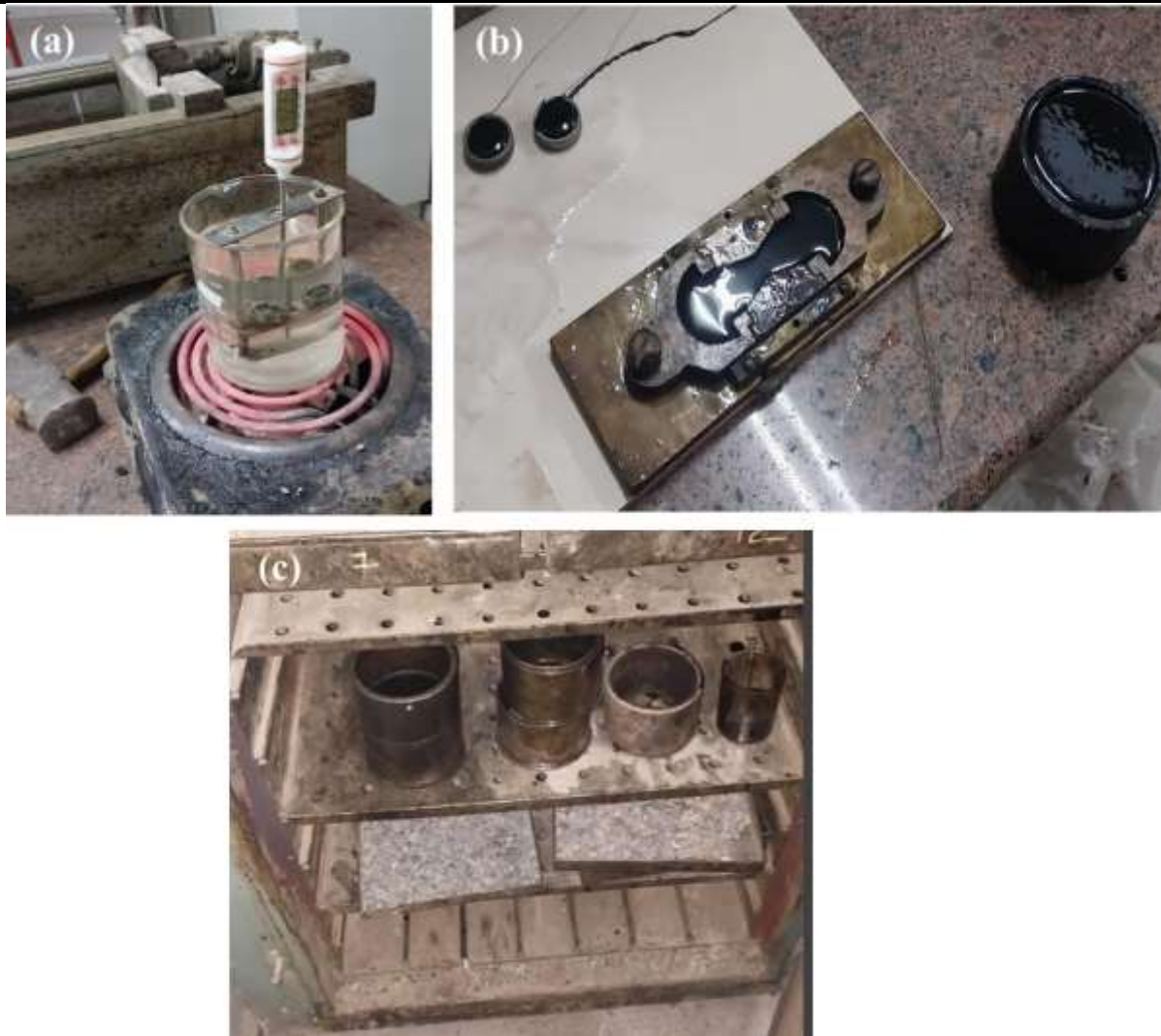
Fig. 2 (a) Softening point Test (b) Ductility setup for Polymer Modified Bitumen (c) Oven used for Drying for Aggregates
