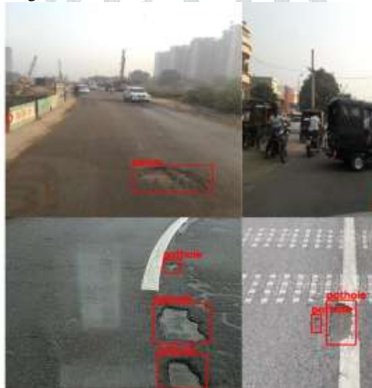
Fig 5.1: Annotated images from the pothole dataset to train the YOLOv8 model on custom dataset.
