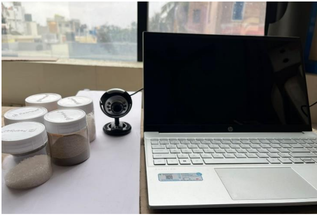
Fig. 8. Computer Vision Setup The setup includes a camera module positioned for optimal ingredient detection and text recognition. The YOLOv5 model processes images in real-time, achieving over 90% accuracy in identifying kitchen items.
