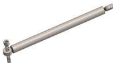
Figure 11: CAD of Adjustable Tie-rod
