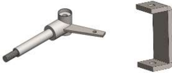
Figure 12: CAD of Steering Knuckle and C-shaped Mount
