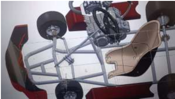
Figure 20: Isometric View of the Kart
