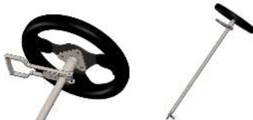
Figure 10: CAD of Steering Column and Wheel
