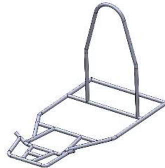
Figure 21: CAD of the Chassis
