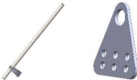
Figure 13: CAD of Pitman Arm & Double Pitman Assembly
