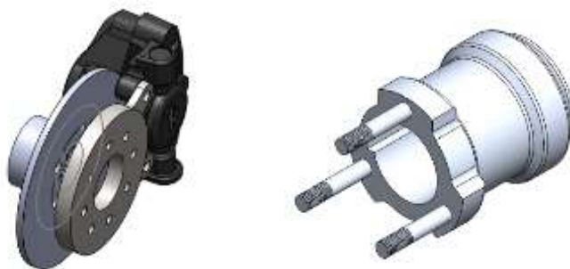
Figure 14: CAD of Front Disk Brake & Hub Assembly
