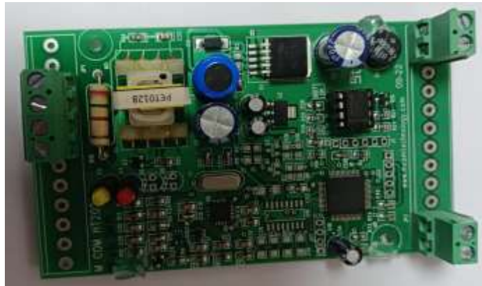
Fig. 4: Hardware Design for HART Converter
