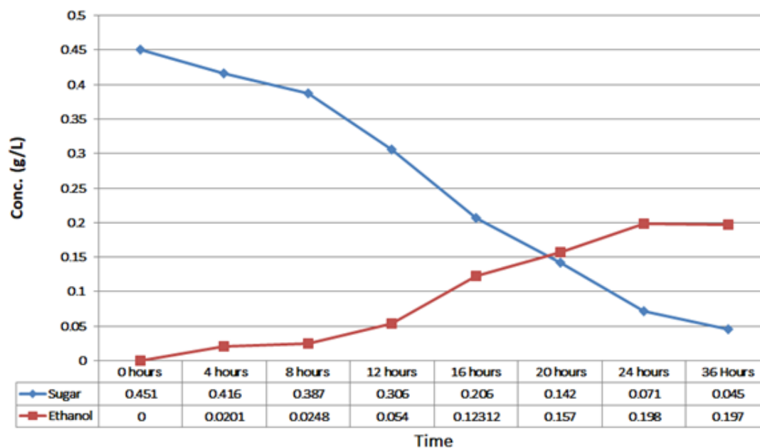
Fig 4: Time Course of Utilization of 3%Reducing Sugar Hydrolysate and Ethanol formation by 0.2% Four Seasons Yeast
