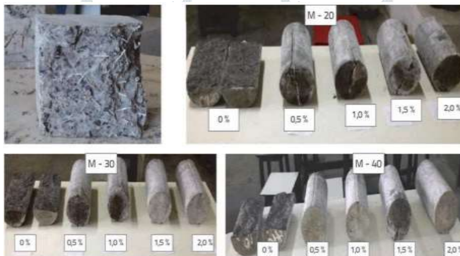
Figure 1.4 Crushed cubes and cylinders containing glass fibers.
