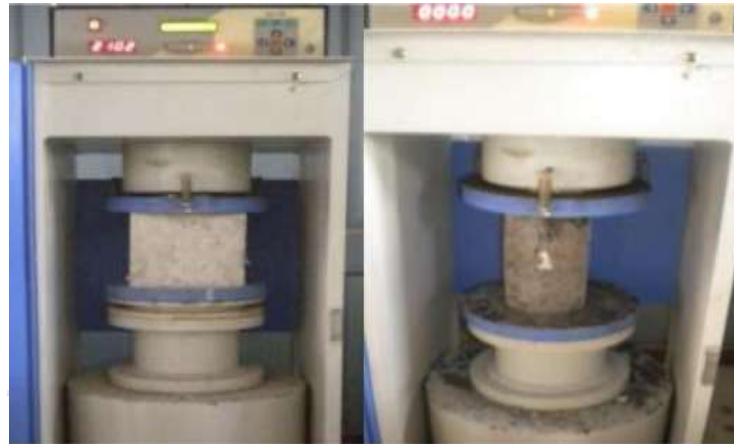
Figure 1.6 Compression test on GFC cylinder
