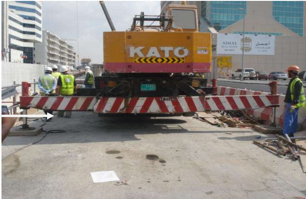
Outrigger not open fully
