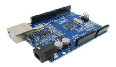
The Arduino uno is an open-source microcontroller which is utilized to control all the devices. The microcontroller board is furnished with sets of advanced and simple information and results ticks that might be communicated to different development sheets and other circuits. The board has 14 info pins and 6 simple info pins. it acknowledges the voltages somewhere in the range of 7 and 20 volts.
