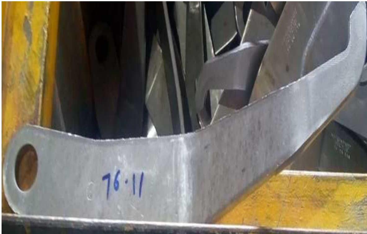
Figure 3.2 Image of Actual Part: Brake Pedal Lever
